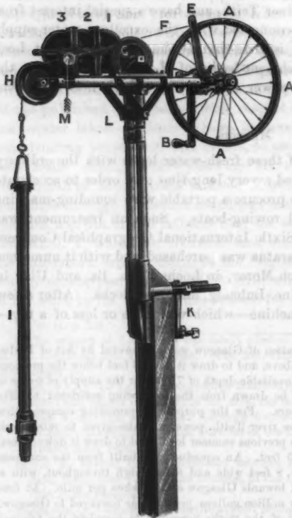
FIG. 1.—F. P. PULLAR'S SOUNDING-MACHINE.
